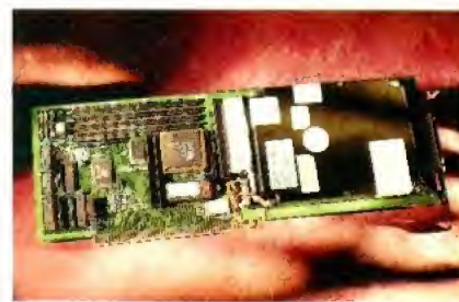
The Trifecta is a rather useful SCSI expansion card for any Zorro-compatible machine.
